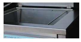
It is recommended to maintain a distance of 100 to 150 mm between the workpiece and the tank walls for proper ultrasonic diffusion. Upon purchase of this ultrasonic cleaning machine, a user and maintenance manual will be provided, including detailed information about the equipment. The content of this document is for guidance only and does not establish any contractual commitment. It may be modified without prior notice to optimize the quality and service offered.
